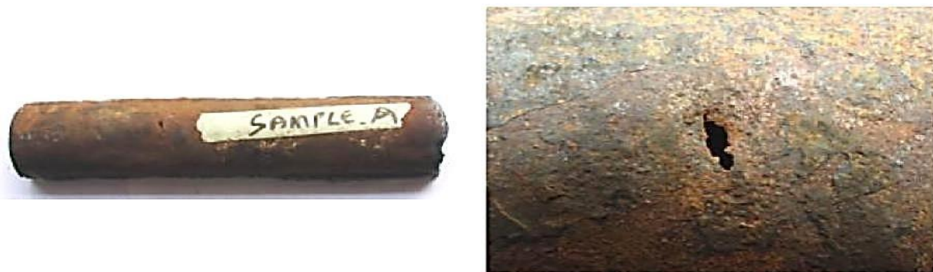
Figure 2: Tube Sample-A obtained from Furnace side for Investigation
