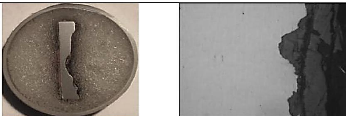
Figure 13: Tube Sample-A specimen in a mounted condition with observed thinning of ID due to pitting like corrosion damage. The unetched view at ID showing corrosion damage with scaling indicating the gouging nature of corrosion damage.
